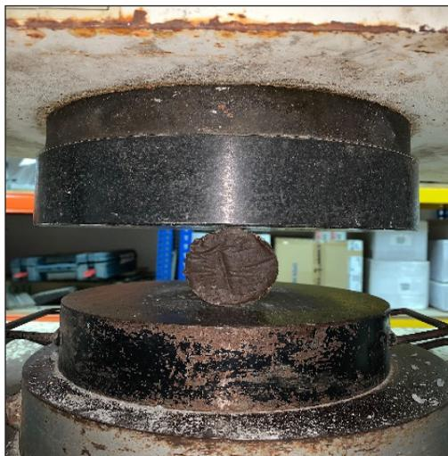
Figure 7. Splitting tensile test
