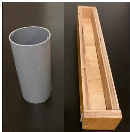
Figure 3. Example of cylindrical and prismatic mould
